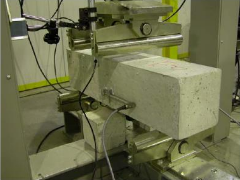
(b) Figure 4. UNI test: (a) geometry and test set-up; (b) specimen image during testing.
